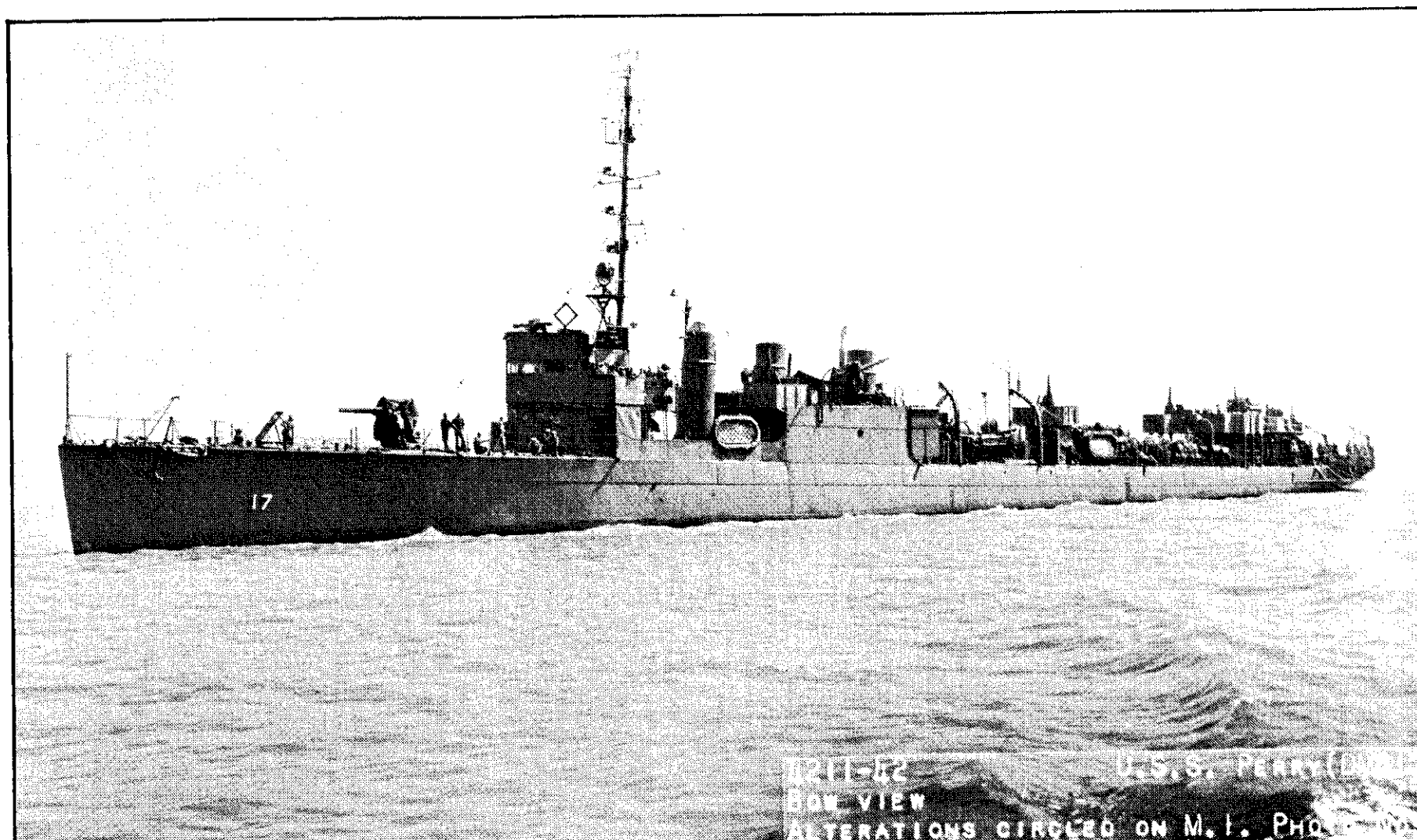
The fast minesweeper U.S.S. Perry (DMS-17) at the Mare Island Navy Yard, California, on July 22, 1942, after changes had been made in her armament to provide better antiaircraft protection. When the Japanese attacked Pearl Harbor on December 7th, 1941, the Perry was able to open fire on enemy planes only when they came within range of her machine guns (six .50-caliber and two .30-caliber). After this attack she patrolled the waters around Hawaii for six months and then returned to the States. Following her 1942 refit the Perry participated in the Aleutian campaign for a year, conducting minesweeping operations, performing rescue missions and acting as a convoy escort. (Official U.S. Navy photograph.)
