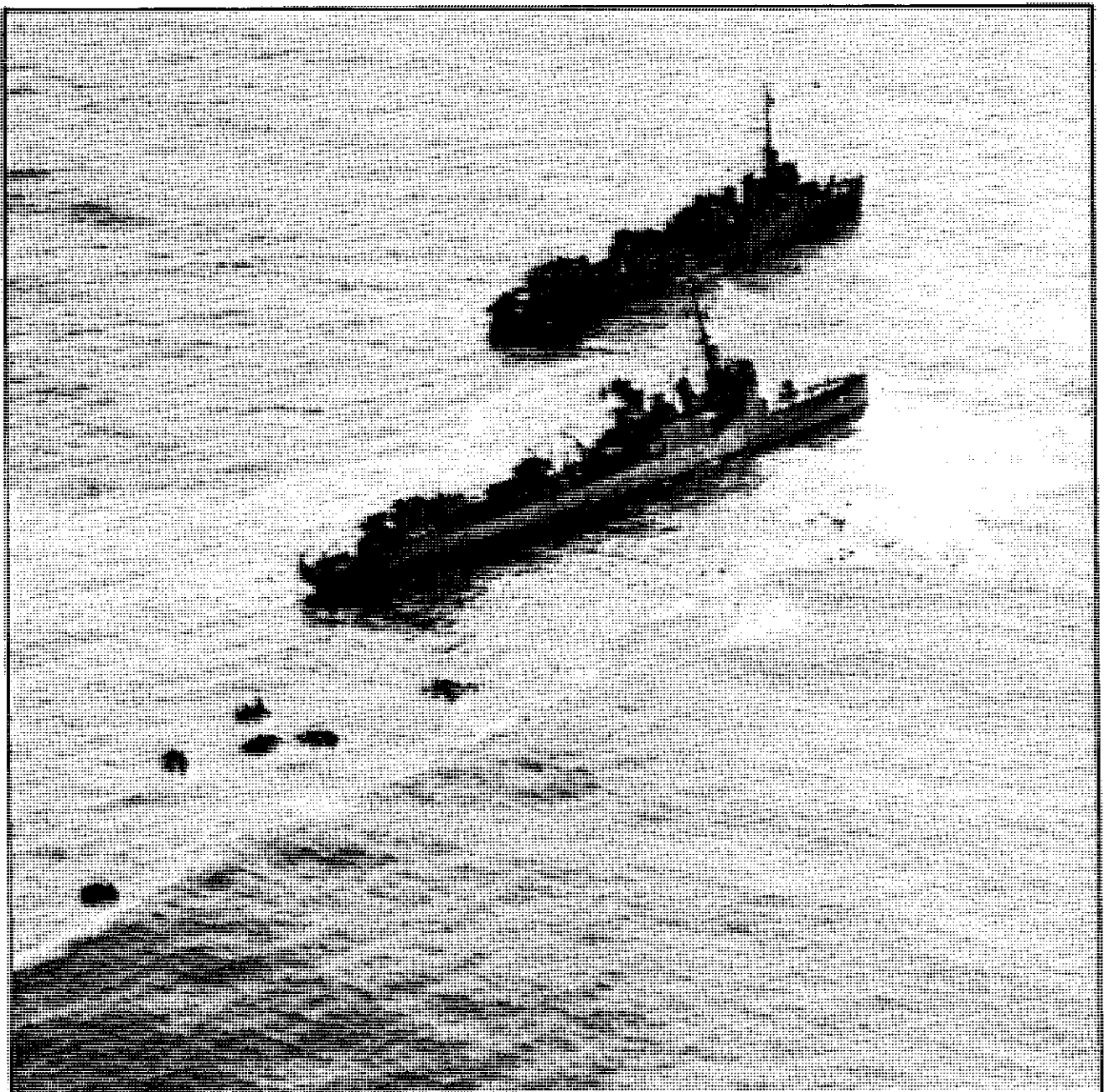
The U.S.S. Parry (DM-17) (center) and the U.S.S. Preble (DM-20) shortly after the Parry was mined on 13 September 1944. The explosion caused an immediate 30 degree list to port and the loss of all power. Both fire-rooms flooded at once, causing the commanding officer, Lieut. William M. Lindsey, USNR, to order "Abandon Ship" just two minutes after she struck the mine. The ship broke in two and sank an hour and forty-five minutes later. Fortunately, casualties were low; 6 killed and 17 wounded out of a complement of 154. This photograph was taken from a floatplane off of the battleship U.S.S. Tennessee (BB-43). (Naval Historical Center)
