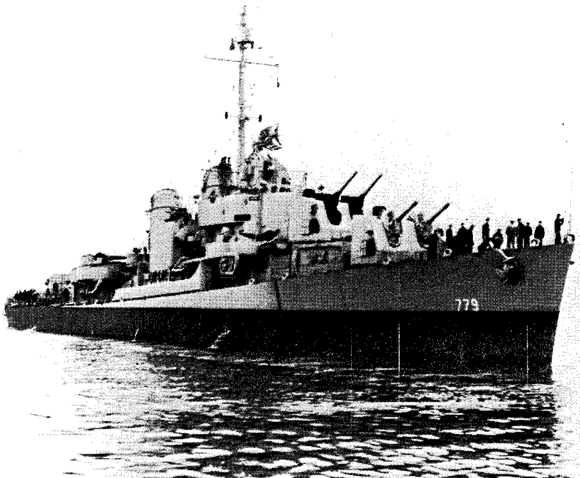
The 2,200-ton Allen M. Sumner -class destroyer USS Douglas H. Fox (DD-779) off the Puget Sound Navy Yard, Bremerton, Washington, on March 15, 1945. Each of the 5-in./38 dual-purpose guns in the twin mounts shown could fire 15 rounds/minute with a well-trained guncrew. These guns fired 55-lb. projectiles with a maximum range of about 9 miles. Note the Measure 22 camouflage: lower hull in Navy Blue and all above in Haze Gray. (Naval Historical Foundation print)
