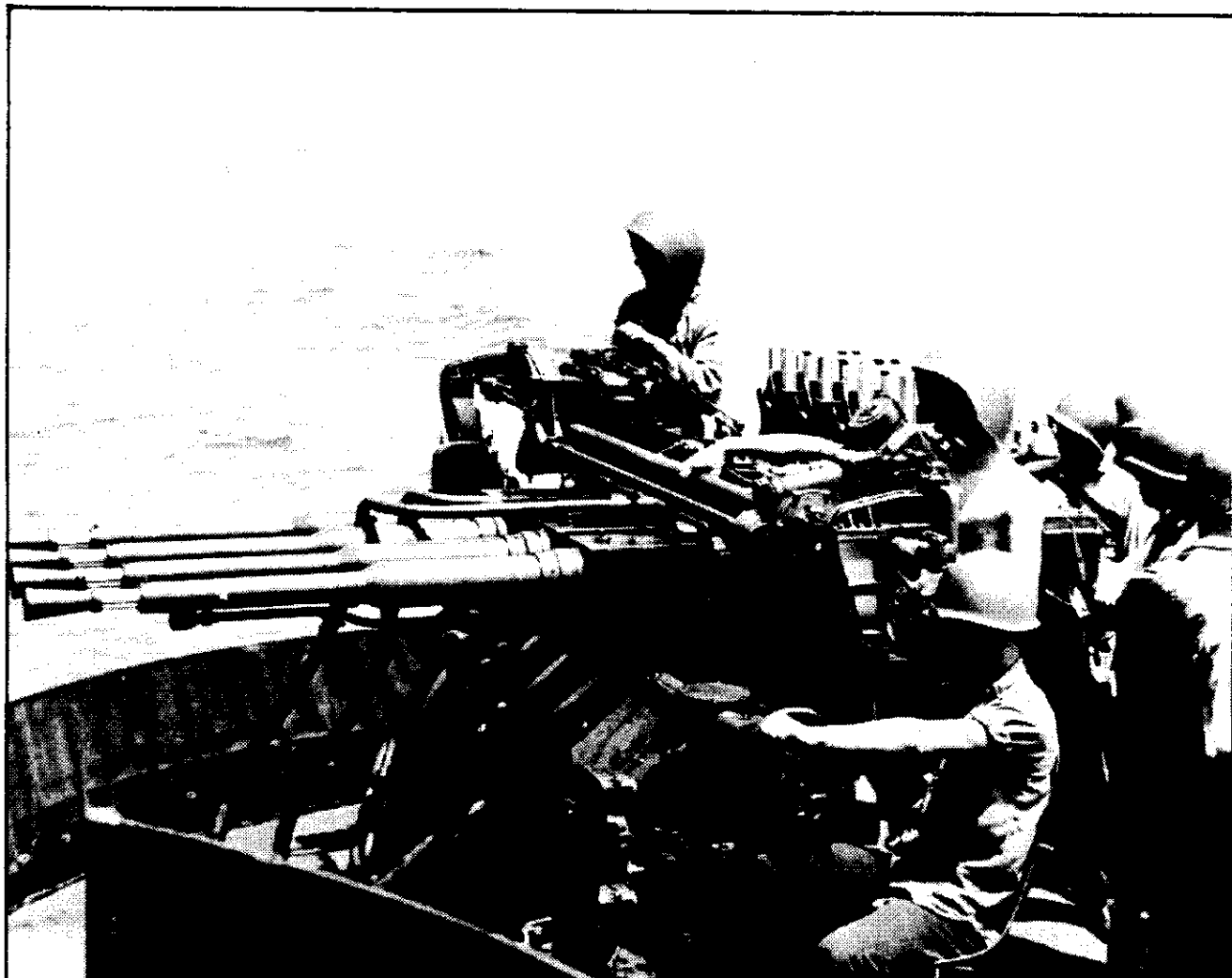
This view of a quad 1.1-inch/75 machine gun/cannon on a destroyer escort shows what the mount on the starboard side of the Duncan's after gun platform looked like. (It was balanced there by a 20-mm Oerlikon machine gun/cannon to port.) Dubbed as the "Chicago Piano" for the way it fired, this medium-range antiaircraft weapon was replaced on U.S. destroyers in 1942-43 with the much more effective 40-mm Bofors automatic gun, in single, twin and quadruple mounts. The "one point ones" could fire 150 one-pound high explosive shells per minute per barrel. Ammunition in 8-round clips was passed up from below through two rectangular scuttles in the deck called "slots." Although this weapon was difficult to maintain and unreliable in use, around 1,000 of them were built before production ended in 1943, and some remained in use aboard older ships and auxiliaries until the war ended in 1945. (Official U.S. Navy photograph.)
