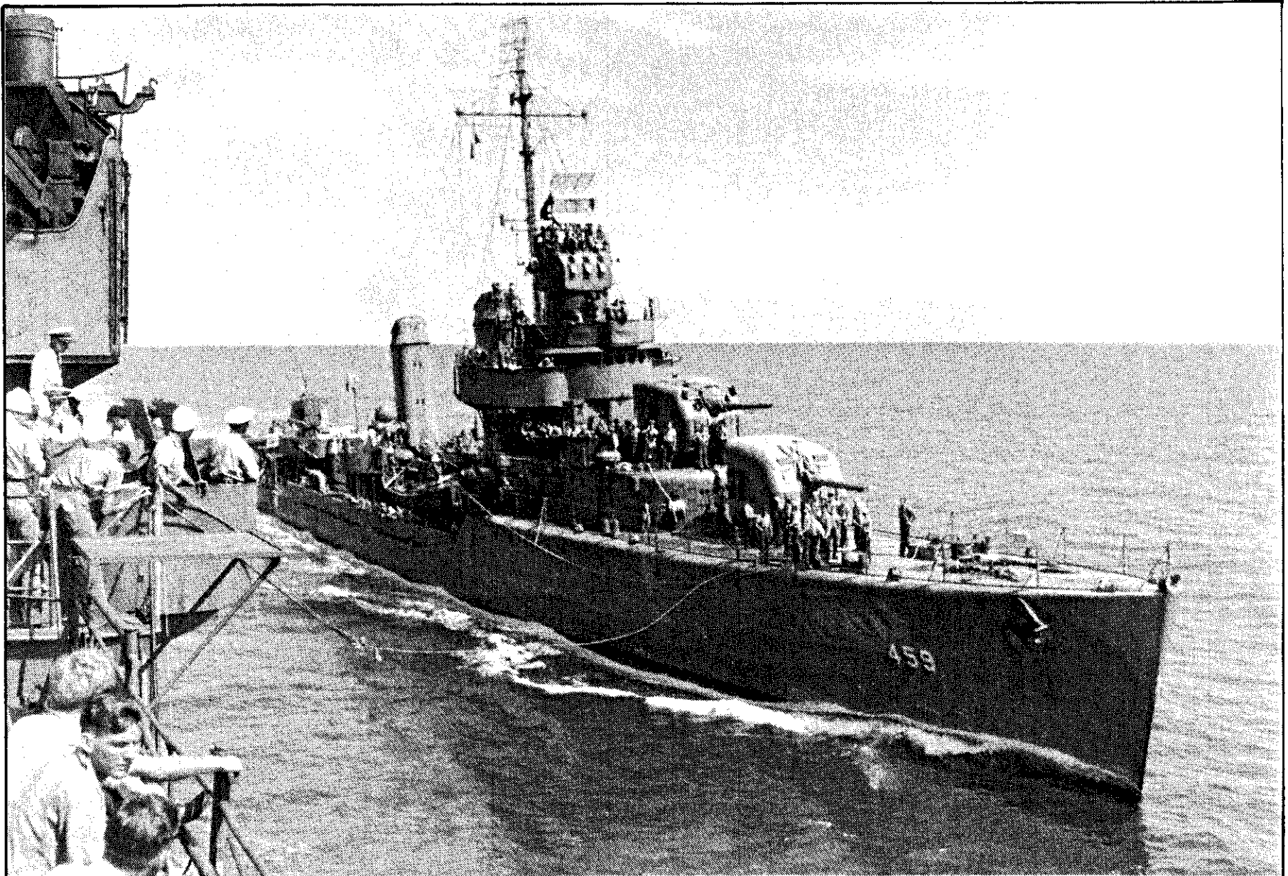
The U.S.S. Laffey (DD-459) (LCdr. W. E. Hank) alongside the heavy cruiser U.S.S. San Francisco (CA-38) to exchange mail while under way on 4 September 1942. This uncensored view of the Laffey shows a Mk 4 fire-control radar antenna mounted on a Mk 37 main gun director over her pilot house and an early SC-type air-search radar antenna atop her foremast. Two days later the Laffey joined up with Task Force 18 (RAdm. L. Noyes) and became one of the screening ships for the aircraft carrier U.S.S. Wasp (CV-7). (USN photo.)
